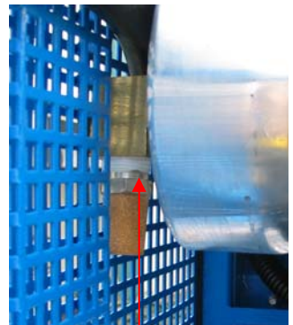
Fixed Factory Set Nitrogen Discharge
