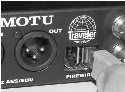
Figure 4-1: Connecting the Traveler to the computer.
