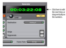
Figure 11-2: Setting the time code start time.
