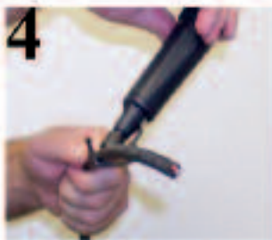
4. Rotate cable stripper 2-3 times around jacket.
