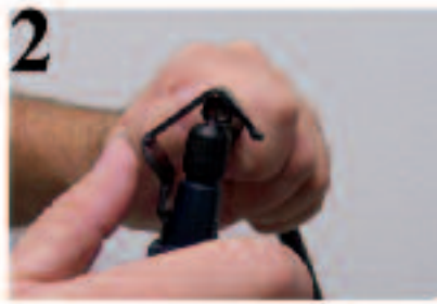
2. Check blade depth before stripping jacket.
