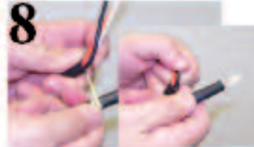
8. Use center of jacket piece to wrap ripcord around jacket piece.
