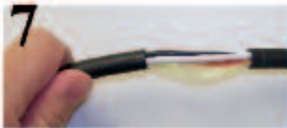
4. Rotate cable stripper 2-3 times around jacket.
