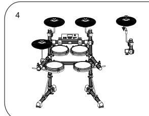
Next, assemble the two cymbals and the hi-hat as shown in the image on the left and tighten their T-screws. If you prefer to have the cymbals lower, you can relocate the cymbal locking mechanisms below the horizontal support tube that holds the toms and the drum module.
