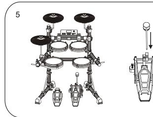
Insert the beater shaft into the beater link of the kick drum pedal as illustrated, and tighten the key bolt with the included key.
