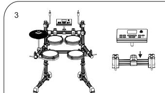
Insert the module into the rack clamp as shown in the figure, and tighten the T-screw.
