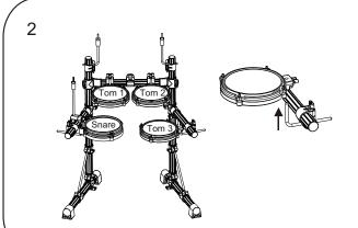
After removing the four pads from the box, insert the pad rod into the pad hole as shown here. Adjust the position of each pad and tighten the screw when you are satisfied.
