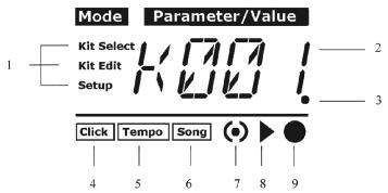
1. Mode This section indicates which mode you are in depending on which of the three options is lit (Kit Select, Kit Edit, or Setup).
