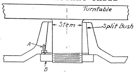
Turntable Revolves on "Stem" and rests on full Diameter Track.
