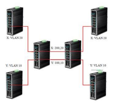
This example shows how to configure switch A with ports 1 on the Switch to tag incoming frames with the service provider's VID of 200 (ports are connected to customer X network) and configure port 7 to service provider's VID of 100 (ports are connected to customer Y network). This example also shows how to set the priority for port 1 to 3 and port 7 to 4.
