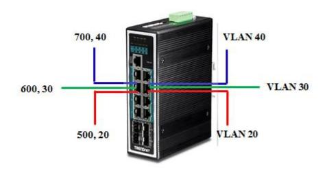
This following example shows how to configure ports 3 on the Switch to tag incoming frames with the different service provider's VID and priority.
