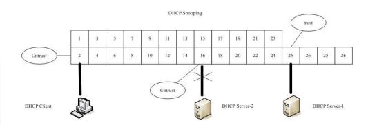
The DHCP server connected to an un-trusted port will be filtered.
