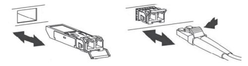
**To properly connect fiber cabling:** Check that the fiber terminators are clean. You can clean the cable plugs by wiping them gently with a clean tissue or cotton ball moistened with a little ethanol. Dirty fiber terminators on fiber optic cables will impair the quality of the light transmitted through the cable and lead to degraded performance on the port.
