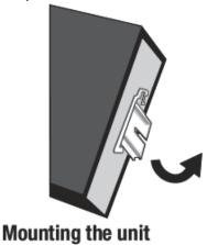
To unmount the switch from the DIN-Rail, slightly pull the switch downwards to clear the bottom of the DIN-Rail and rotate away from DIN-Rail to unmount.
