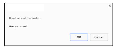
• Click **OK** again and then wait for the Switch to restart. This takes up to two minutes. This does not affect the Switch's configuration.
