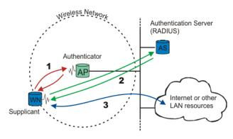
When the client provides the login credentials, the Switch sends an authentication request to a RADIUS server. The RADIUS server validates whether this client is allowed access to the port.
