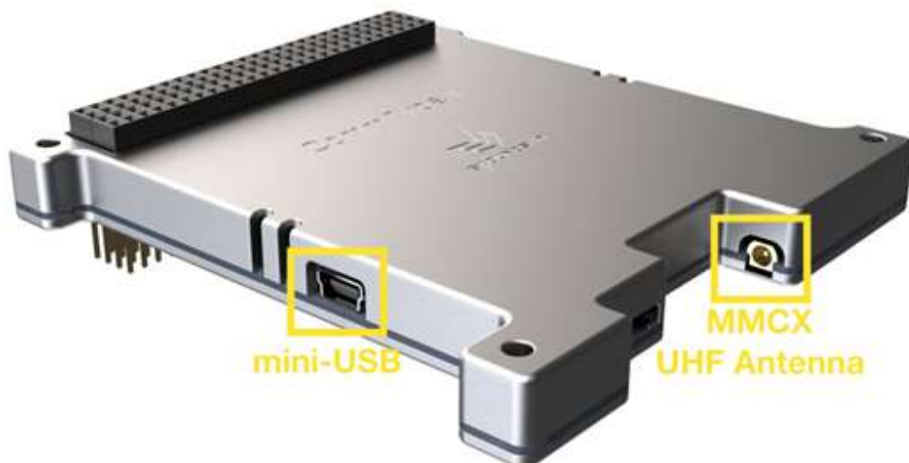
Figure 12: MMCX and Mini-USB Connector Location
