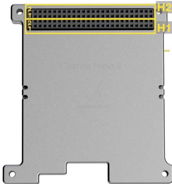
Figure 11: Main Stack Connector Location
