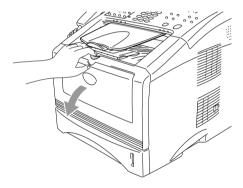
4 Pull out the drum unit and toner cartridge assembly. Pull the jammed paper up and out of the MFC. If you cannot remove the drum unit and toner cartridge assembly easily at this time, do not use extra force. Instead, pull the edge of the jammed paper out of the paper tray. If the jammed paper can not be pulled out easily, turn the jam dial towards you as you gently pull the paper out.
