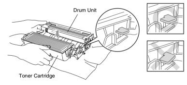
7 Clean the primary corona wire inside the drum unit by gently sliding the blue tab from right to left several times. Return the blue tab to the Home position (▼) before reinstalling the drum unit and toner cartridge assembly.
