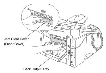
7 Close the jam clear cover (fuser cover). Close the back output tray.
