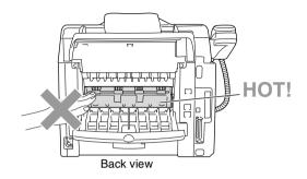
**6** Open the jam clear cover (fuser cover). Pull the jammed paper out of the fuser unit.
