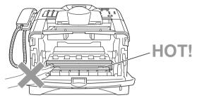
1 Open the front cover and pull out the drum unit.
