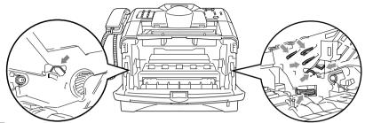
**5** Open the back output tray. Pull the jammed paper out of the fuser unit. If the paper jam can be cleared, go to Step 7.
