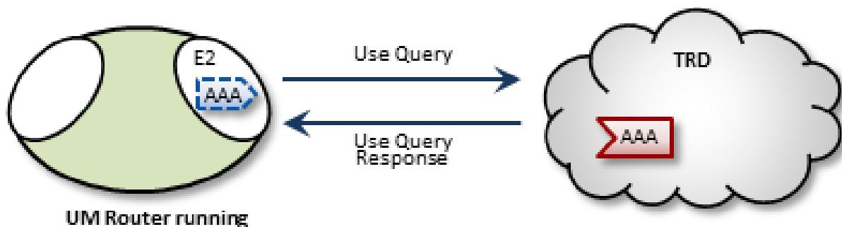
In the case of multi-hop UM Router configurations, UM Routers cannot detect interest for remote contexts via Use Queries or TQRs. They do this instead via Interest Messages. An endpoint portal generates periodic interest messages, which are picked up by adjacent UM Routers (i.e., the next hop over), at which time interest is refreshed.
