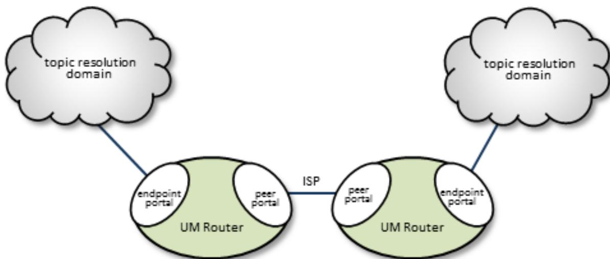
You configure portals in the UM Router's XML configuration file, specifying the portal's name, cost, UM Configuration, Access Control Lists and other attributes. See [XML Configuration Reference](#).
