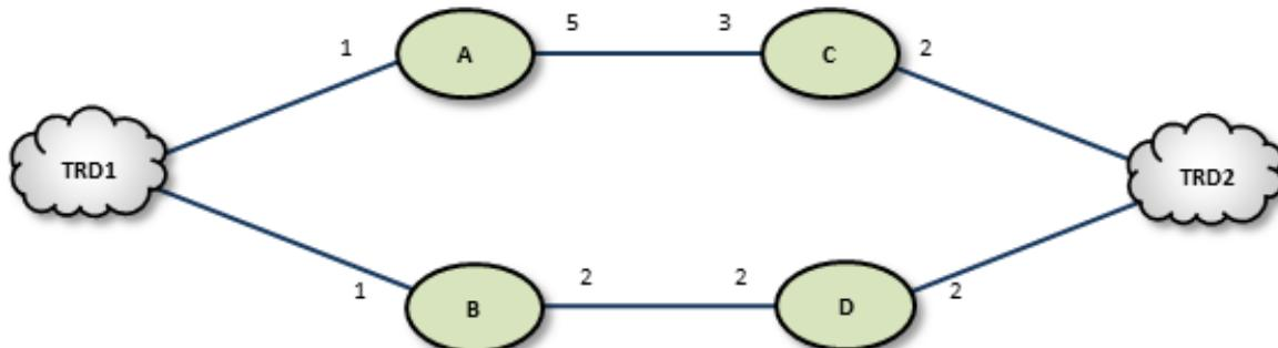
If a UM Router or link along path B-D should fail, the UM Routers detect this and reroute over path A-C. Similarly, if an administrator revises cost values along path B-D to exceed a total of 12, the UM Routers reroute to A-C.
