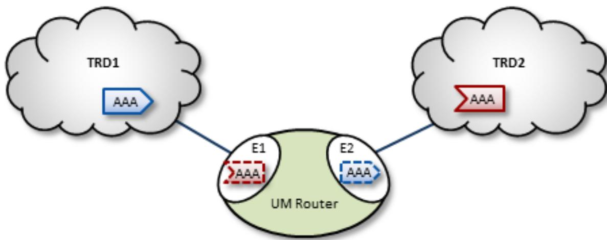
To establish topic resolution in an already-running UM Router, the following sequence typically occurs in an example like the above figure.
