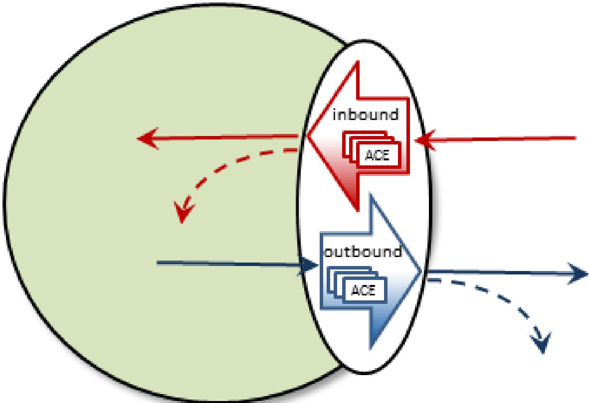
An ACL can contain one or more Access Control Entries (ACEs). ACEs are the filters that let you match (and accept or reject based on), criteria elements. For example, to accept only messages for topic ABC:
