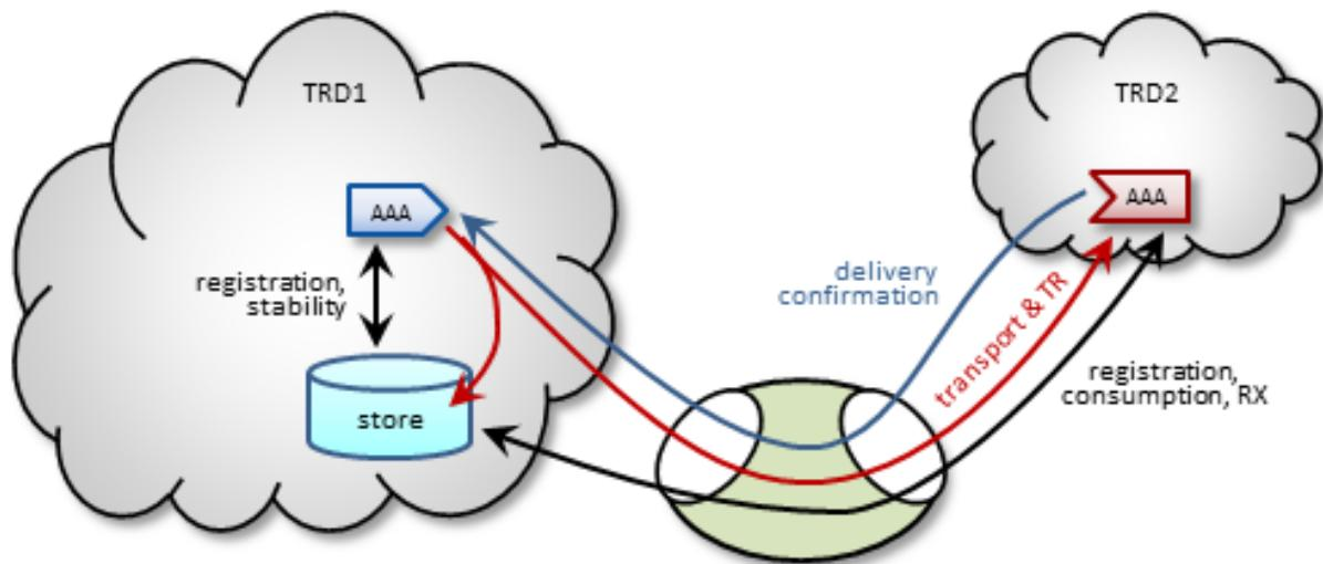
The UM Router also supports UMP implementations with the store located in a receiver's TRD, as shown in the following figure.
