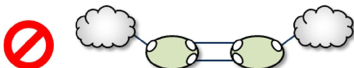
Two endpoint connections from the same UM Router to the same TRD:
