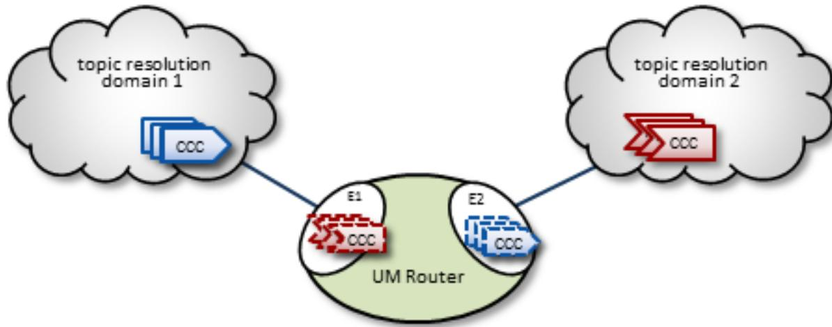
Portals exist while the UM Router is running, however, the UM Router creates proxy sources and receivers during topic resolution and deletes them when the topic is retired.
