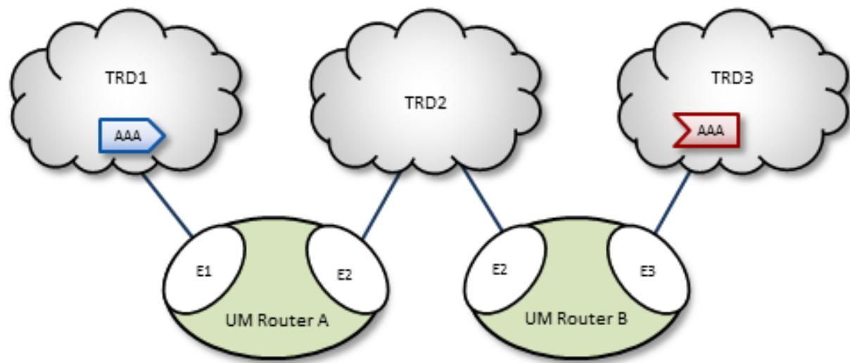
In this diagram, UM Router A has two endpoint portals connected to topic resolution domains TRD1 and TRD2. UM Router B also has two endpoint portals, which bridge TRD2 and TRD3. Endpoint portal names reflect the topic resolution domain to which they connect. For example, UM Router A endpoint E2 interfaces TRD2.
