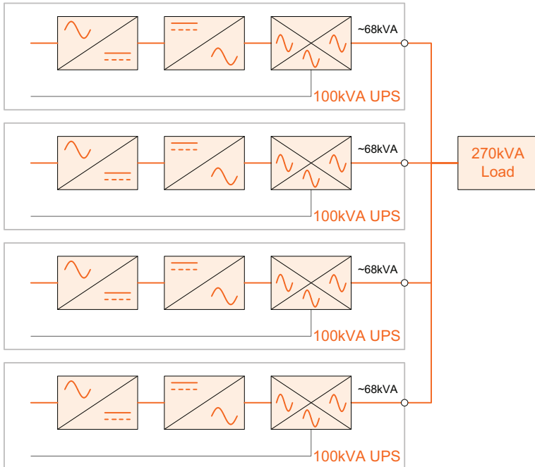
Figure 7.3: Parallel Redundant System
