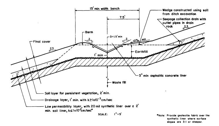
Figure 6-7. Typical run-on control ditch for waste units. 6-17
