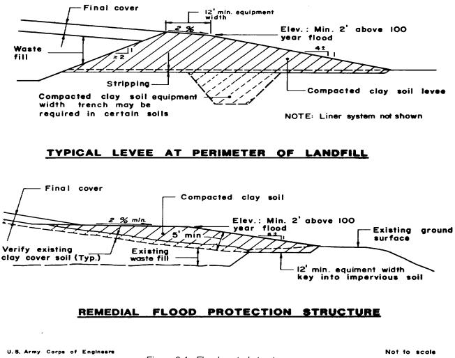
Figure 6-1. Flood control structures.
