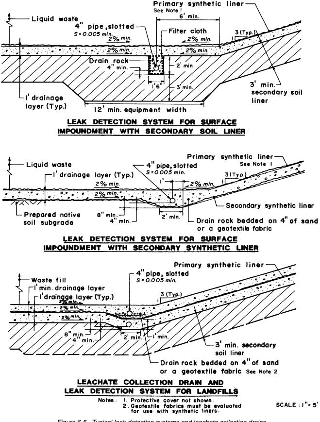
Figure 6-5. Typical leak detection systems and leachate collection drains
