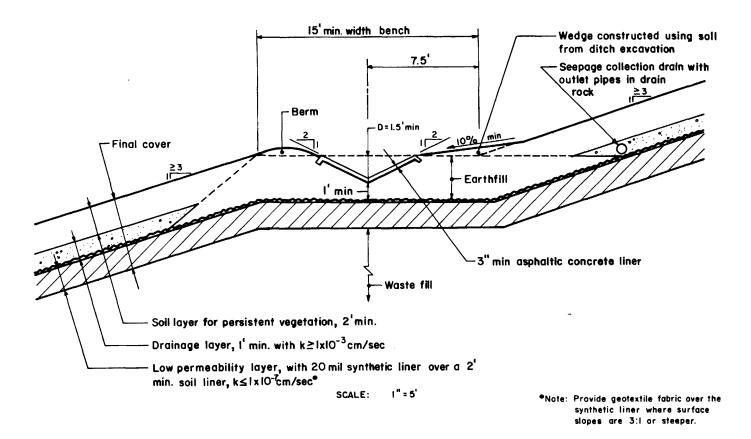
Figure 6-8. Typical run-off control ditch for final cover areas. 6-18
