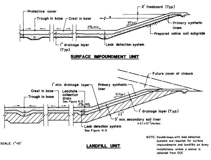
Figure 6-2. Base liner details for landfills and surface impoundments.
