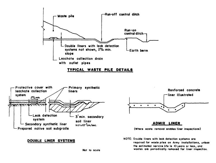
*Figure 6-3. Base liner details for waste piles.* **6-6**
