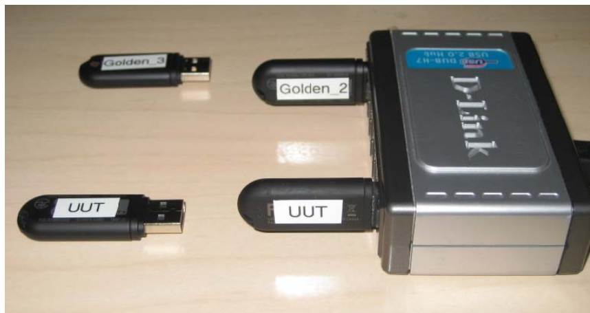
Figure 3b: USB2 golden unit and UUT connected with Hub
