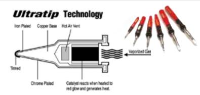
By choosing the tip shape closest to the component you're soldering, and always selecting the largest tip, you'll transfer heat more efficiently at lower settings. We offer a wide selection of tips for your applications.
