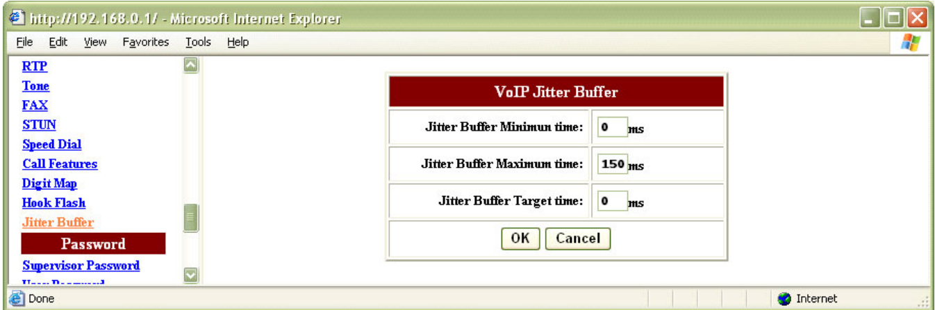
Figure 57 VoIP - Jitter Buffer
