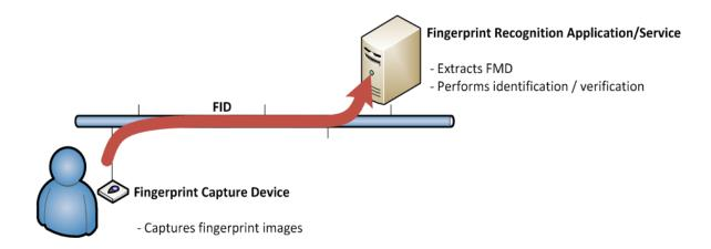
Optionally, the fingerprint capture device can compress the image before transmitting it.
