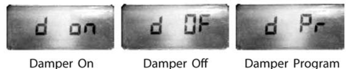
Figure 17: Damper operation and setting.
