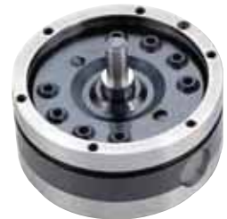
The Model 120 chuck has a reference hole on center (shown here with a step pin). Threaded holes are also provided for mounting the chuck to a baseplate.
