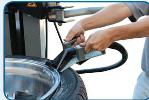
Bead Blaster In Use
