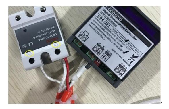
6. use a 2pin cable to connect A1 and A2 of SSR to black terminal of PCB board.
