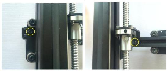
Dismount the BLTouch bracket from left carriage, then assemble the BLTouch sensor as below and mount it back onto the carriage.
