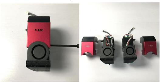
Remove the two screws holding the blower fan.
