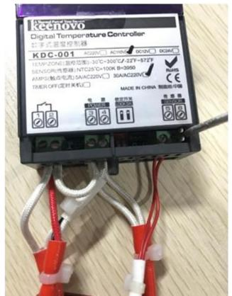
3. connect above two wires to the blue terminal of PCB board.
