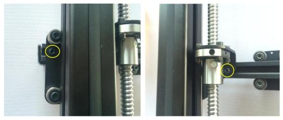
Put aside all components attached to the X axis bar, leaving only the extruded aluminum bar.
