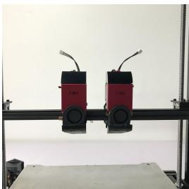
Insert the BLTouch cables into the extruder PCB board.
