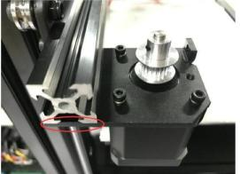
Replace the metal plate on the driven timing belt pulley.
