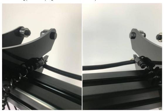
Affix the spring buckle carabiner onto the DB cable using the provided zip ties.
