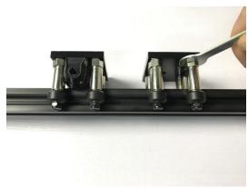
After properly adjusting the carriages, tighten the two screws marked by the blue arrows, below.
