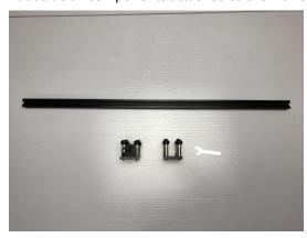
Install the new carriages onto the X axis bar. **Alternate** a few times between the nuts on the same carriage as you tighten them in order to make sure that the wheels are snug against the bar.
