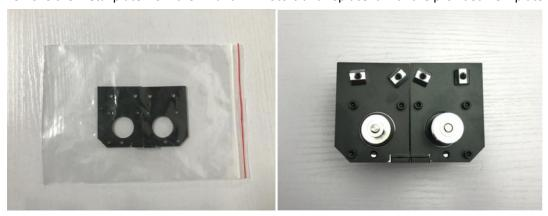
Re-install the motors onto the X axis aluminum bar. The edge of metal plate and the end of the aluminum extrusion should be flush.
