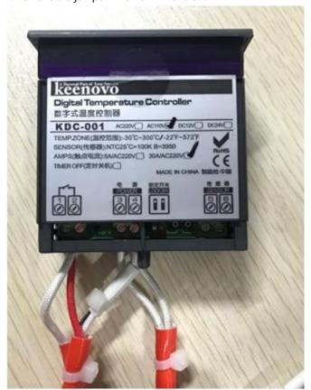
5. Take out two cables from 1# and insert them into the L1 of SSR. Then take out the cable from 3# and insert it into the T1 of SSR.
