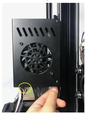
Install the wire guides onto the frame as shown below, then connect the two DB cables.
