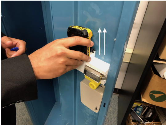
Figure 16: Pulling Off the Battery
