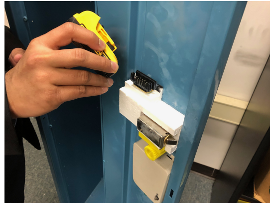
Figure 17: Removal of the Battery
