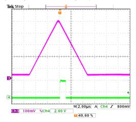
**SCA8:** The green trace shows the output of an SCA, in this case SCA 8. It is produced by a pulse with a peak amplitude within the SCA range (set in software). Its rising edge is at the time the peak is detected. Its width is commandable to 0.1 or  $1~\mu s$ .
