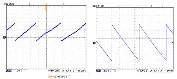
**Preamplifier output.** These traces also shows the preamp output but on a different voltage and time scale to illustrate the reset. The small steps from each signal integrate towards the rail, where a reset signal is generated. This results in a sawtooth of several volts amplitude. The period depends on the total current through the detector (signal current plus leakage current). The plot on the left (right) is for a FastSDD® with PA210, that on the right for a Si-PIN with an XR-100.
