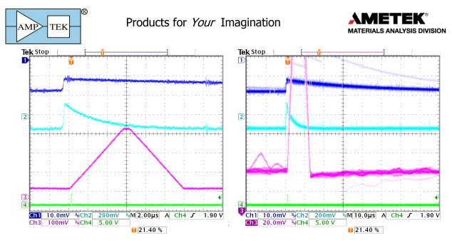
**Pole zero correction**: The traces above show signals from a detector with resistive feedback, in this case an HPGe detector with a 50  $\mu$ s tail. The dark blue trace, the preamp output, drops exponentially to baseline rather than exhibiting the steps of the reset preamplifier. Circuitry in the DP5 cancels this tail (known technically as pole-zero cancellation) so that the light blue trace exhibits a strictly exponential recover, yielding the magenta trapezoid.
