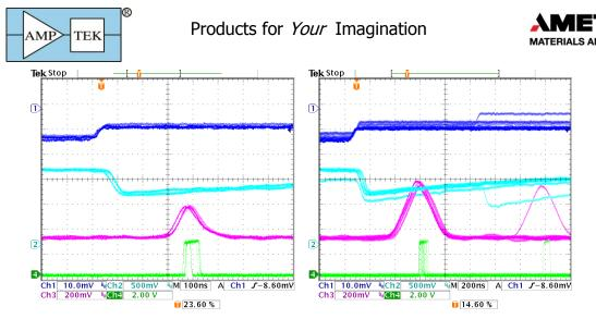
ICR: These traces illustrate the ICR (Incoming Count Rate) pulse. This is produced by a comparator operating on the fast channel. Any pulses which exceeds the fast threshold will generate an ICR pulse. This is used to produce the fast or input count rate and in the pile-up reject logic.
