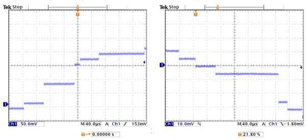
**Preamplifier outputs.** These traces illustrate typical output pulses with Amptek's X-ray detectors, which use reset preamps. The plot on the left is for a FastSDD® detector; each X-ray interaction results in a positive going step of ~3.7 mV/keV. One can distinguish the 5.9 and the 22.1 keV steps. The plot on the right is for a Si-PIN, which produces negative going pulses with a gain of 1 mV/keV.
