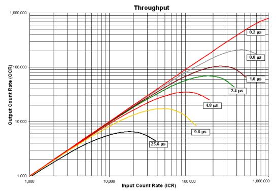
If  $R_{in}$  is the input count rate,  $R_{out}$  is the output count rate,  $T_{peak}$  is the peaking time, and pile-up rejection is enabled, these curves follow closely the equation
