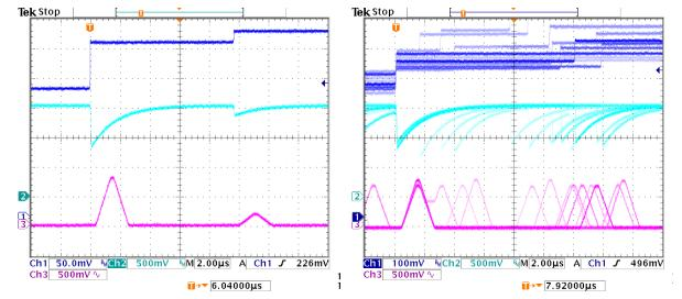
**Signals.** These traces show the preamplifier output (dark blue), the input to the ADC (light blue) and the shaped output (magenta) for typical pulses. The shaped output is on the DAC output. The trace on the left shows two pulses which are well separated in time. The plot on the right shows several pulses, illustrating the random timing and occasional pulse pileup.
