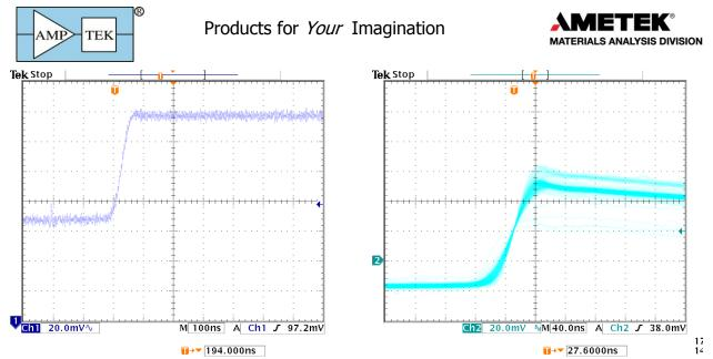
**Preamplifier risetime**. The plot on the left shows the trace from the preamplifier for a single pulse at a short time scale, while the trace on the right shows the input to the ADC from several pulses. These are for a FastSDD® with  $^{55}$ Fe. The distinct traces for the  $K_{\alpha}$  and  $K_{\beta}$  energies are visible.
