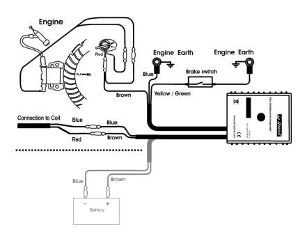
The Xtra.CDI Shutdown Transponder has two cables on the transponder. A CDI based engine does not supply enough energy to power the transponder and has a different electrical signal then conventional engines.
