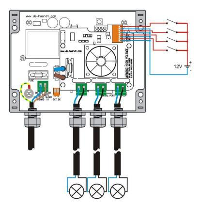
In the picture above there is given an example wiring for the 4 external control input signals. The table below describes the functions of the 8 pins of the external input connector.
