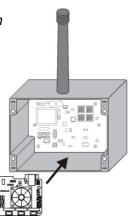
When positioning the Light Control Board on the Xtra.Range extender board, be sure that the pin header on the Range Extender board is on the same position as the connector on the backside of the Light Control Board.
