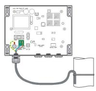
Standard the Xtra.Range Extender is supplied with a 230V mains power cord.
