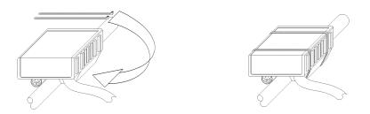
Fasten the Xtra.CDI Shutdown Transponder with 2 tie wraps, and ensure that these cannot tremble off during the use of the kart or by other causes.
