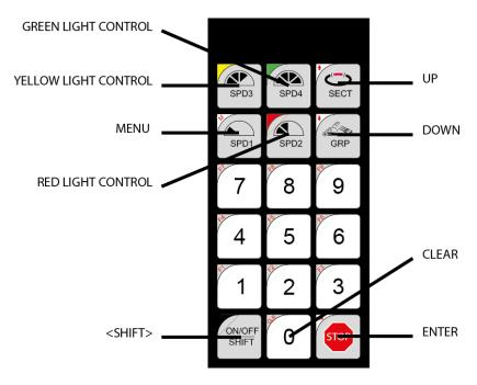
Press the **ON/OFF** button on the keyboard of the Xtra.Remote Control for at least one second to turn the device on. Once on, you can do the same to turn it off.
