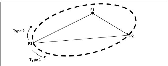
The bold dashed line above represents the elliptic conic section that connects P1 and P2. We see that the lower transfer arc between P1 and P2 only covers about 90 degrees, and so it is Type 1. The upper transfer arc covers about 270 degrees, and so it is Type 2.
