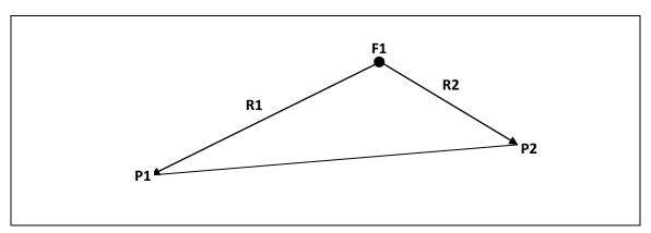
Given two points P1 and P2 with position vectors from F1 known as R1 and R2, respectively, and two different times T1 and T2, the goal in solving Lambert's problem is to find the solution to the differential equation
