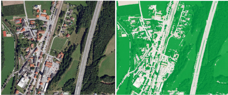
Figure 2.3. An image for analysis displayed in Pixel View, next to the same image in Classification View. The colors in the right-hand image have been assigned by the user and follow segmentation and classification of image objects
