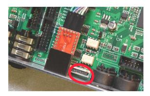
Insert two jumpers supplied with Drawbar Controller to jumper header PL18 on positions 7-8 and 9-10 as shown in picture. Connect 5-wire MIDI cable (supplied) to HX3 MIDI Expander MIDI IN/OUT and to HX3 Drawbar Controller MIDI OUT. HX3 Drawbar Controller will now be phantom powered by the HX3 MIDI Expander through the MIDI cable.
