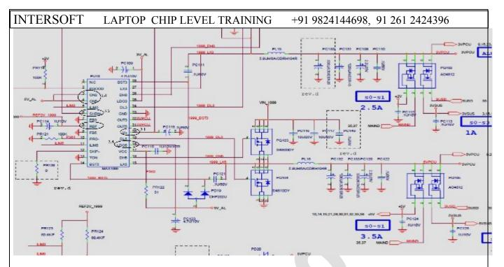
Fig. System power main 5v 3v generate max 1999 schematic diagram
