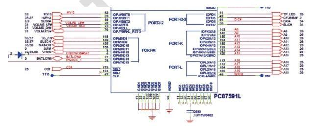
South Bridge received DNBSWON low, it occurs SUSB #, SUSC # 2 high sent to 97551/87591, South Bridge chip part of the line is always in working confition. Likewise, it is also connected to a 32.768kHz Y5, its role is to South Bridge chip modules RTC and basic detection module reference clock.
