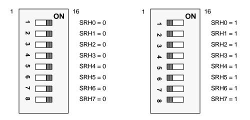
Figure 1-2. General-Purpose Software-Readable Header
