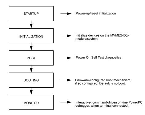
Figure 2-1. SYSTEM BOOT-UP SEQUENCE
