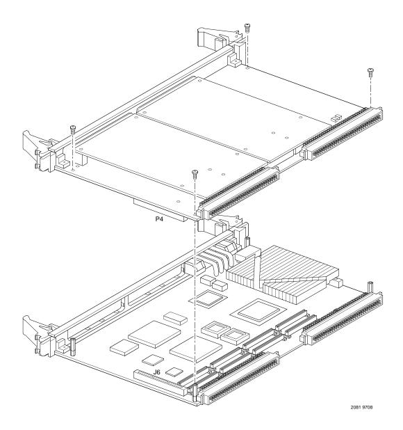
Figure 1-4. PMCspan-002 Installation on an MVME2400x
