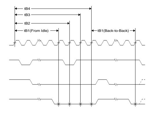
Figure 3-2. Timing Definitions for PPC Bus to SDRAM Access
