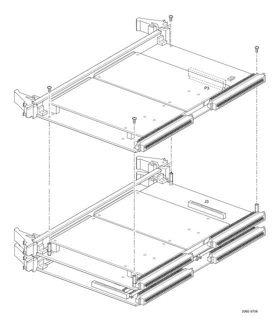
Figure 1-5. PMCspan-010 Installation on a PMCspan-002/MVME2400x
