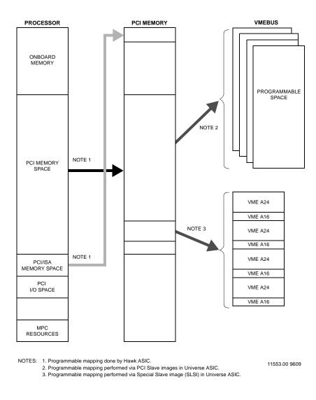
Figure 4-1. VMEbus Master Mapping
