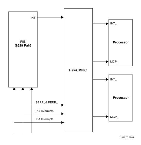
Figure 5-1. MVME2400 Series Interrupt Architecture
