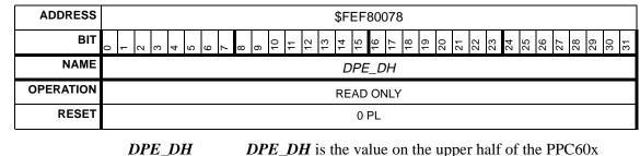
\_DH DPE\_DH is the value on the upper half of the PPC60x data bus at the time of the last logging of a PPC60x data bus parity error by the Hawk. It is updated only when dpelog goes from 0 to 1.
