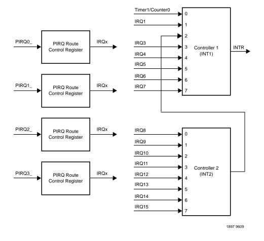
The following figure shows the interrupt structure of the PIB.
