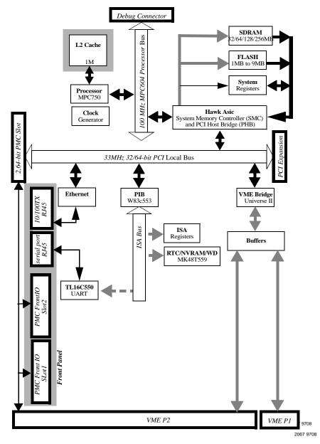
Figure 1-1. MVME2400 Series System Block Diagram
