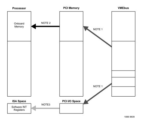
Figure 1-3. VMEbus Slave Mapping
