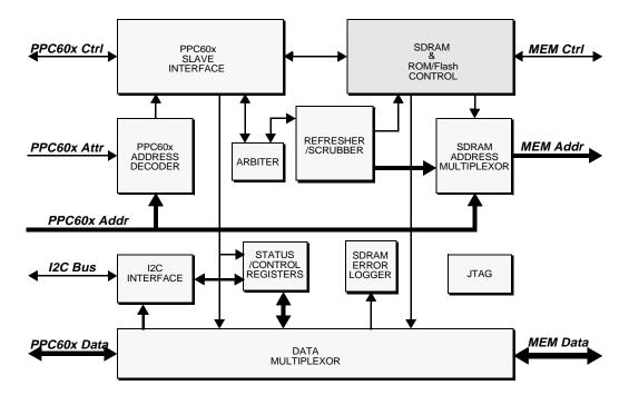
Figure 3-4. Hawk's System Memory Controller Block Diagram
