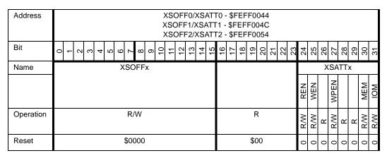
The <u>PPC Slave Offset Registers</u> (**XSOFF0, XSOFF1, and XSOFF2**) contains offset information associated with the mapping of PPC memory space to PCI memory/io space. The field within the XSOFFx registers is defined as follows:
