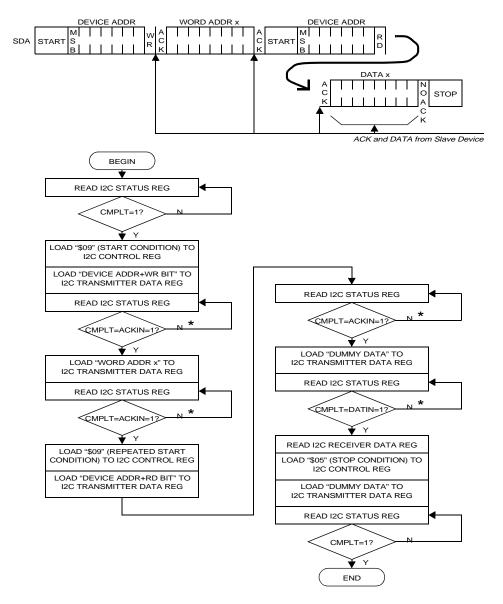
(\*): Stop condition should be generated to abort the transfer after a software wait loop (~1ms) has been expired
