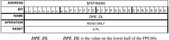
*DL DPE\_DL* is the value on the lower half of the PPC60x data bus at the time of the last logging of a PPC60x data bus parity error by the Hawk. It is updated only when *dpelog* goes from 0 to 1.
