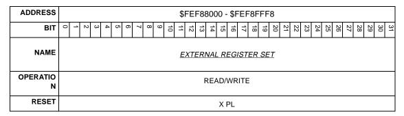
**EXTERNAL REGISTER SET** The **EXTERNAL REGISTER SET** is user provided and is external to the Hawk. It is enabled only when the **tben en** bit is cleared. When the **tben en** bit is set, the **EXTERNAL REGISTER SET** is disabled and the Hawk does not respond in its range except for the tben register at \$FEF88300.
