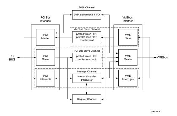
Figure 4-1. Architectural Diagram for the Universe II
