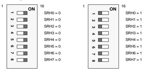
Figure 1-4. General-Purpose Software-Readable Header
