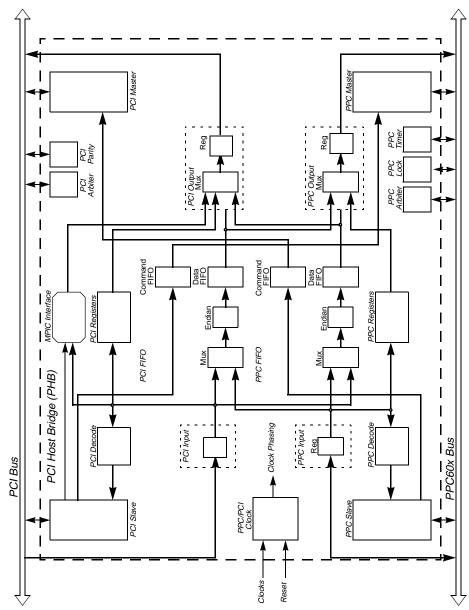
Figure 2-1. Hawk's PCI Host Bridge Block Diagram
