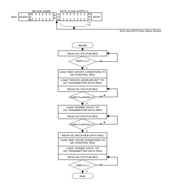
(\*): Stop condition should be generated to abort the transfer after a software wait loop (~1ms) has been expired
