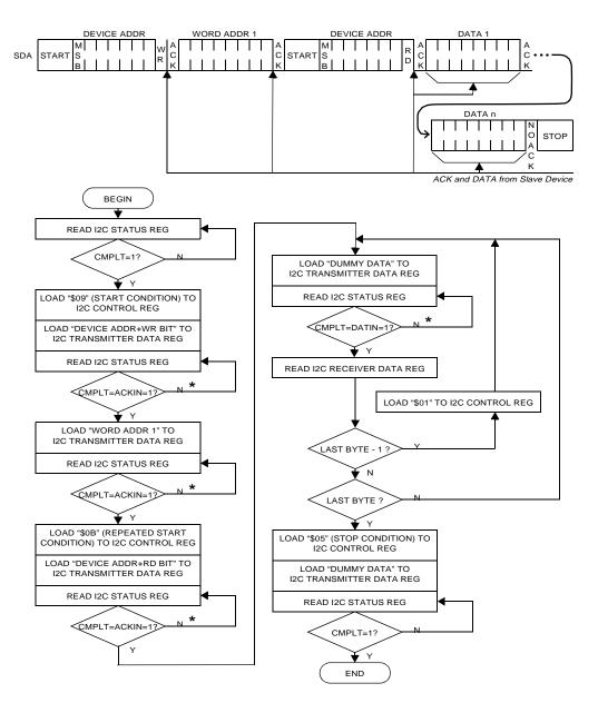
(\*): Stop condition should be generated to abort the transfer after a software wait loop (~1ms) has been expired
