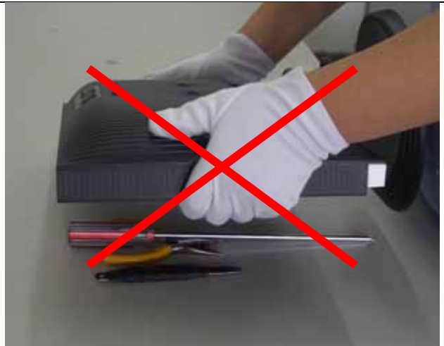
The panel is placed facedown on the lap. That may cause "Mura."
