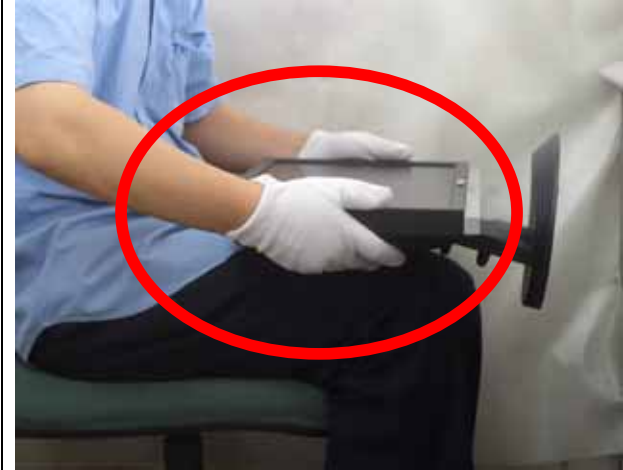
Place the monitor on the lap, the panel surface must be upwards.
