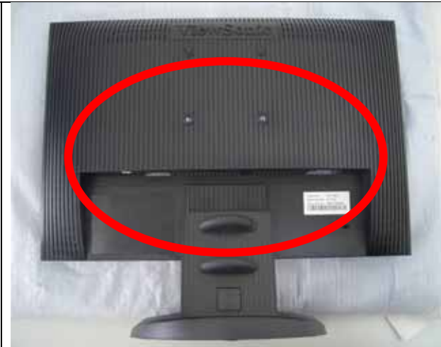
Place the monitor on the lap, the panel surface must be upwards.
