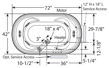
Product Shown: Venicia™ Whirlpool Bath Right Hand Shown Model: EJ00 \* Measurements inside unit represent cutout in floor to allow for drain/overflow. Minimum Service Access dimensions given.
