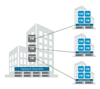
Virtual SAN 2 Node configurations are Virtual SAN Stretched Clusters comprised of two data nodes and one witness node. This is a 1+1+1 Stretched Cluster configuration. Each data node behaves as a data site, and the two nodes are typically in the same location. The witness VM could reside at the primary datacenter or another location.
