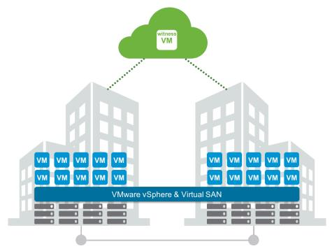
Each site is configured as a Virtual SAN Fault Domain. The nomenclature used to describe a Virtual SAN Stretched Cluster configuration is X+Y+Z, where X is the number of ESXi hosts at data site A, Y is the number of ESXi hosts at data site B, and Z is the number of witness hosts at site C. Data sites are where virtual machines are deployed. The minimum supported configuration is 1+1+1 (3 nodes). The maximum configuration is 15+15+1 (31 nodes).
