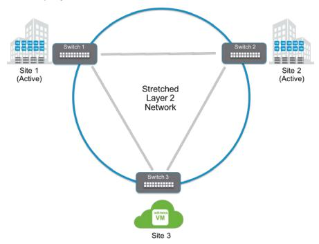
In the event of the link between Switch 1 and Switch 2 is broken (the link between the Site 1 and Site 2). Network traffic will now route from Site 1 to Site 2 via Site 3. Considering VMware will support a much lower bandwidth for the witness host, customers may see a decrease in performance if network traffic is routed through a lower specification Site 3.
