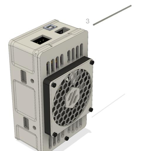
**Step 4:** Screw in the M3 8mm screw through the door and into the brass insert at the bottom of the case. This is the lock for the RAMPs case and will keep the door closed during operation.
