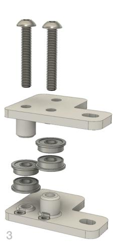
**Step 3**: Assemble the idler bearing stacks and secure the assembly using the 2 M5 30mm cap
