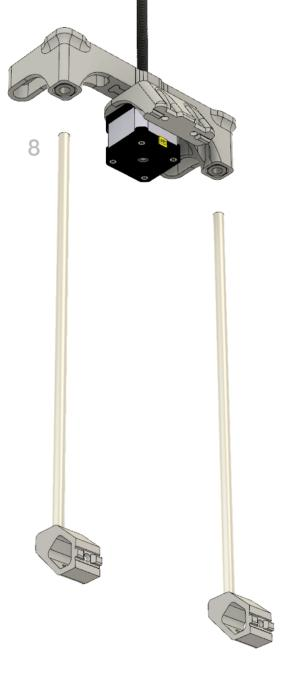
**Step 8:** Insert both 8mm shafts into the bed carriage bearings and cap the shafts with the upper Z shaft supports.
