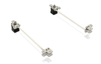
**Step 1**: Clean out the motor mount holes and secure the motors to the A and B motor mounts using the M3 8mm socket screws. Use the neoprene washers on both sides of the motor mount. This will provide vibration isolation during printer operation. Make sure the motor wires are facing **away** from the Y shaft retainer, as pictured.
