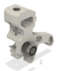
**Step 2:** Insert a 625 bearing into the retainer on the flat portion of the extruder body.
