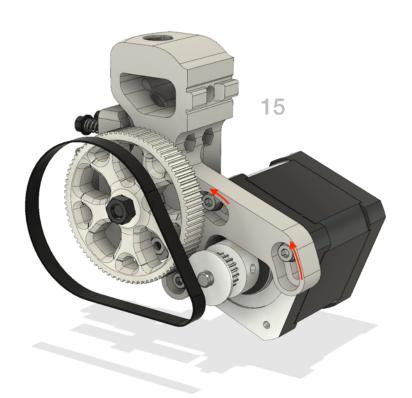
**Step 15:** Twist the motor towards the front of the extruder, and slip on the GT2 belt loop.
