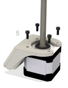
**Step 5:** Secure the Z motor mount to the lead screw motors using 4 M3 8mm screws.
