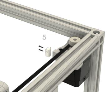
**Step 5:** Attach the Y end stop switch (the one with the longer wire) to the A motor mount.
