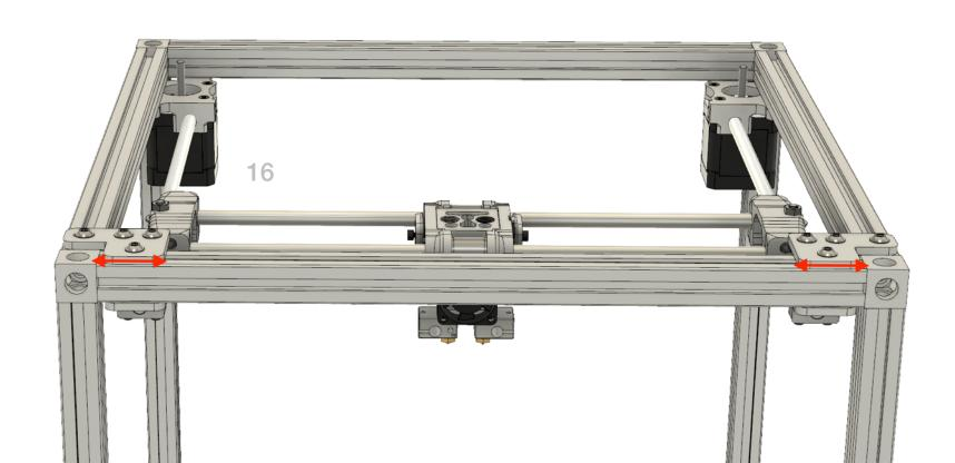
**Step 17:** Check the gantry for racking. When pushed all the way forward it will be obvious to see a difference in gaps. While the front XY Joint retainer screws are loose, you can tweak the X axis to make fully perpendicular to the Y axis.
