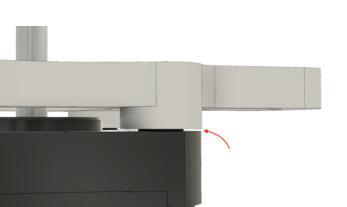
**Mind the gap:** When tightening the socket screws, make sure there is still a visible air gap between the motor and the mount.
