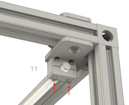
**Step 11:** Tighten the Y shaft retainer screws on both sides.
