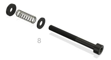
**Step 8:** Use a steel M3 washer, a spring, and a M3 nylon washer to assemble a tension bolt as illustrated. You'll need 2 of them.
