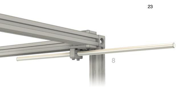
**Step 8:** Insert both 8mm Y shafts half way into their retainers on the idlers.
