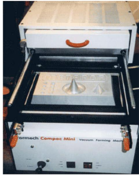
Fig. 5.4 A metaphor mould demonstrated on one of the Formech range of vacuum forming machines
