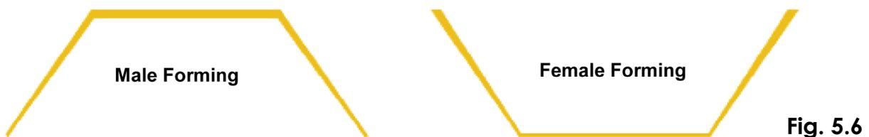
A greater degree of definition is achieved on the side of the plastic in contact with the mould. The choice of a male or female should be considered so that the side requiring the highest definition is the one in contact with the mould especially thicker plastics.
