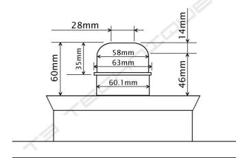
Keep in mind that there are three sizes of grease caps that came on Vanagons. By far the most common is 35mm in height. The tallest version (rare) is about 55mm tall and the rest are 43mm in height. It is possible to shorten the 35mm grease cap by approx. 5mm if needed for centercap clearance. The 43mm grease cap could be shortened by 13mm.
