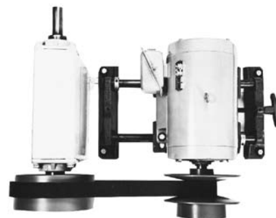
Adjustable Center V-Flat Drive Minimum Speed Position
