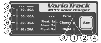
authorized by the initial settings of the equipment. The equalization phase will be authorized as from the beep after having pressed the key « Set » (4) for 2 seconds. The « Charge » light indicator flashes 3x as long as the equalization phase is not completed. The equalization can be interrupted by pressing a second time for 2 seconds: a double beep indicates that the function has been cancelled. The indicator (2) stops flashing 3x confirming the cancellation.
