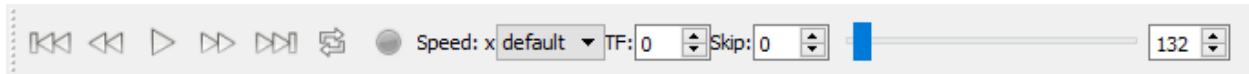
Figure 15 : playback control tool bar. From left to right : Go to start, Go previous frame, Start / Stop, Go next frame, Go to end, Loop, speed, Trailing frame, Skip and Select frame slider.
