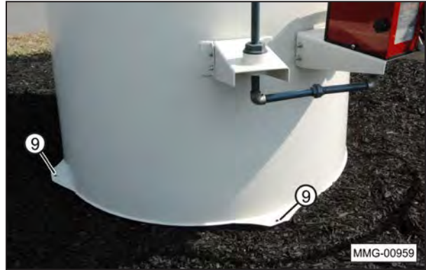
(9) Fuel Tank Anchor Points.
