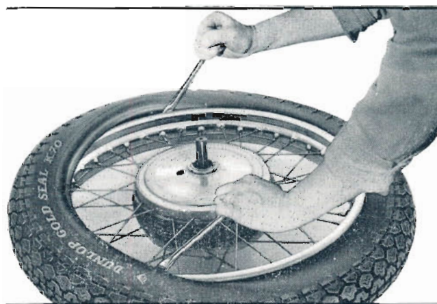
FIG. F.23. Removing the first bead.
