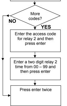
This code will be used to open the door/gate (Relay 2). The code can be from 4-8 digits long and must be different from the engineer's code.
