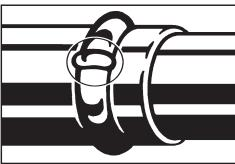
When the fitting is pressed (Figure 1.3), a permanent, sealed, non-detachable, mechanical connection is created.
