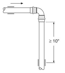
At no point in the piping system should a fitting be the sole means of support. For example, when installing a tee, both the branch and the trunk must be properly supported. Piping systems should be isolated from shock and vibration through the proper use of hangers, supports and vibrationeliminating devices.
