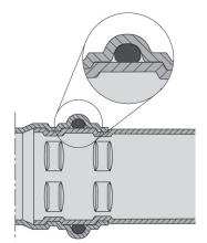
Viega fittings are pressed before, after and on top of the sealing element in a single step, which creates a permanent connection that is secure and guaranteed to last.
