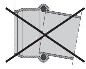
Fittings that do not have cylindrical pipe guides risk making an unsecure connection. Without the pipe guides, installers can possibly damage the sealing element.
