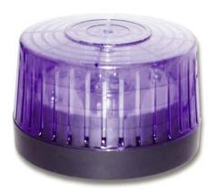
The SL-2 is a 360° LED Strobe and/or Beacon visual indicator. LED's not only are more efficient and last longer than standard flash tubes but are also immune to shock and vibration. The LED's are internally positioned to allow a 360° viewing angle when the unit is mounted vertically and a 120° viewing angle when side mounted.
