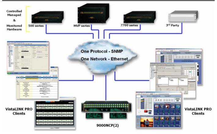
Figure 1-1: VistaLINK® Architecture
