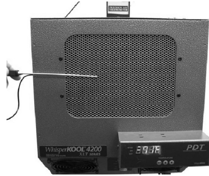
OUTLET AIR -- Evaporator (Front) Side*
