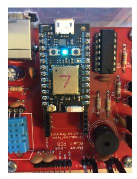
There is another LED on the right side of the board. When working properly the blue LED will blink on/off every five seconds.
