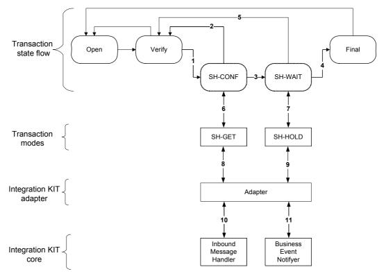
TRMSwift uses two modes to process a business event. The first mode indicates which transaction is picked up for processing (SH-GET in the example). The second mode is used to find the transaction again so that it can be updated with the status of the sending of messages (SH-HOLD in the example).
