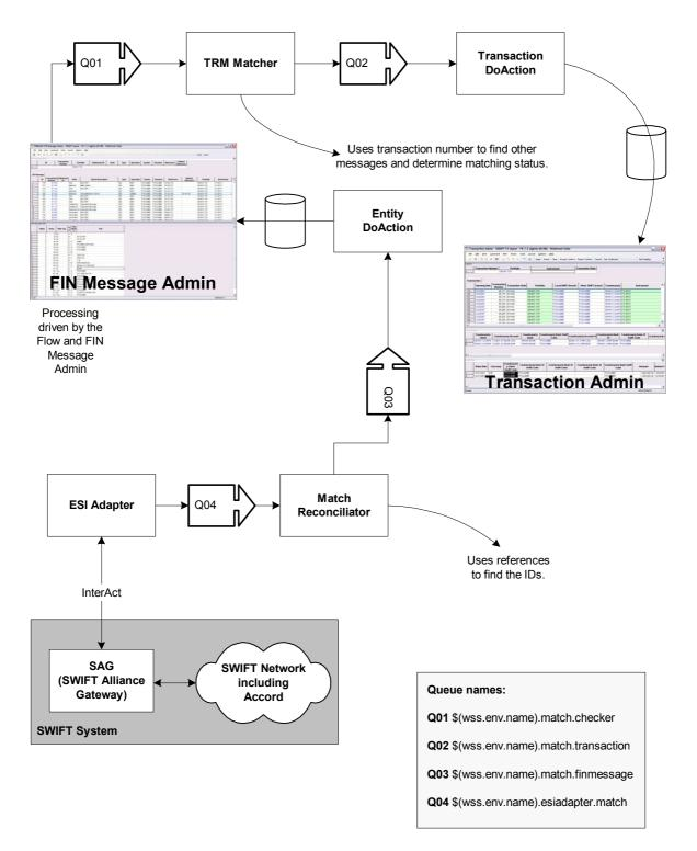
ESIadapter compiles a query for the BIC in question according to the ESICRM Editor, and sends the request for information to Accord. This request (query) and matching status (query result) are based on the API definition. Once a matching status is returned from Accord, it is made available for further processing on an incoming queue (Q04). At this point, the references in the matching status are the references used in the FIN messages that had previously been sent to SWIFT.
