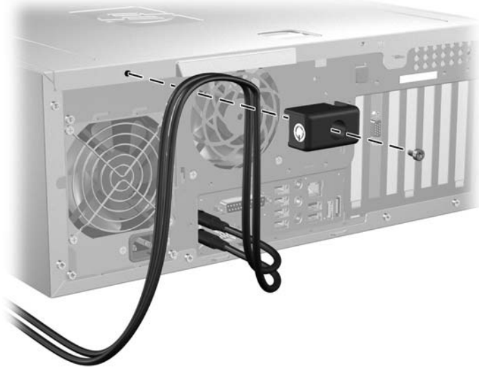
Figure 4-6 Removing the lock screws
