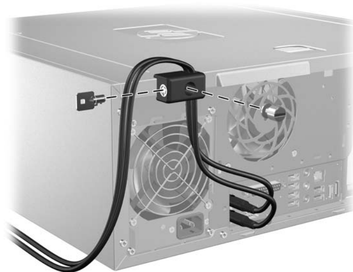
Figure 4-5 Unlocking the device
