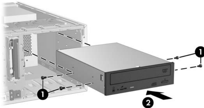
Figure 4-44 Installing the optical drive
