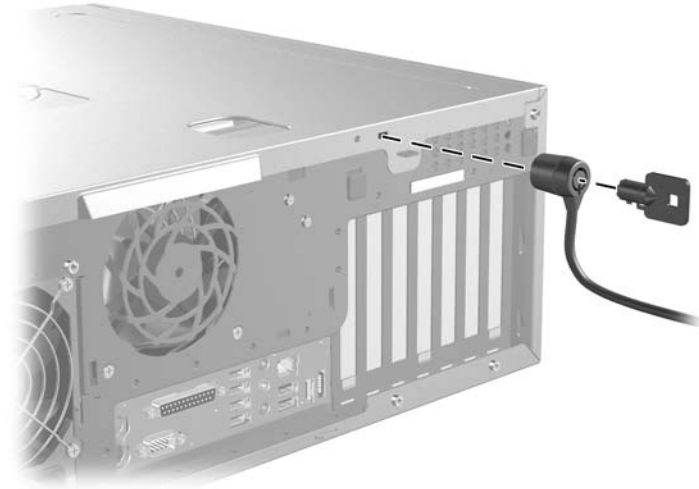
Figure 4-4 Removing the cable lock
