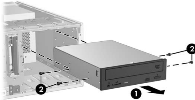
Figure 4-43 Removing the optical drive screws
