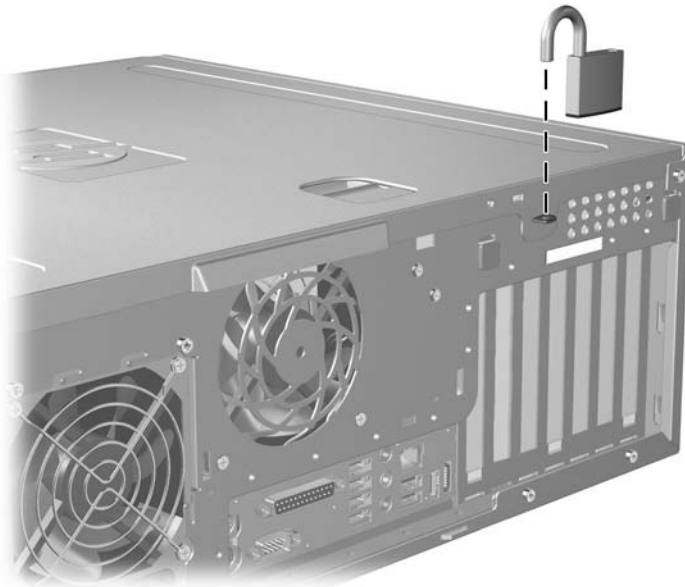
Figure 4-3 Removing the security lock
