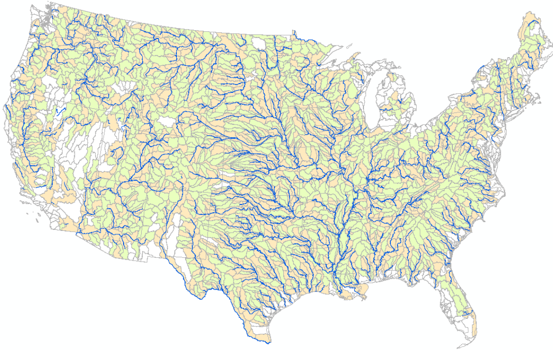
Figure 3. River network (blue lines) connecting 8-digit HUC watersheds of the conterminous US.
