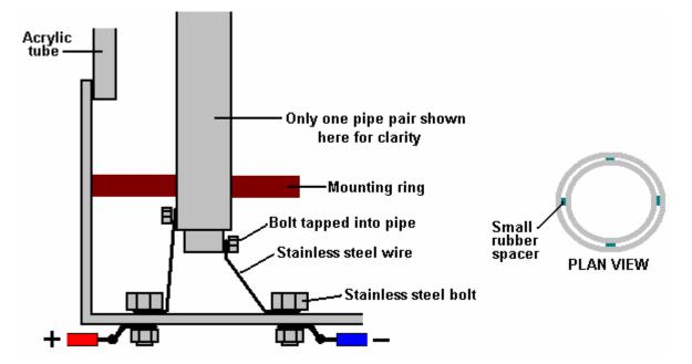
The bolts tapped into the inner tubes should be on the inside and the bottom of the two tubes aligned in spite of them being spread out as shown above. The diagram shows the inner connection on the outside, only for clarity. The bolts going through the base of the unit should be tapped in to give a tight fit and they should be sealed with Sikaflex bonding agent or some similar waterproofing material.
