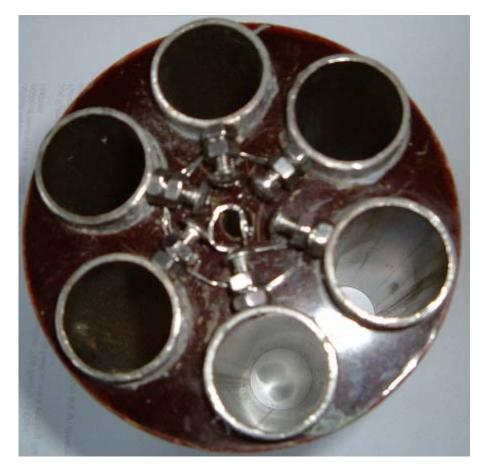
The electrical connections to the pipes are via stainless steel wire running between stainless steel bolts tapped into the pipes and stainless steel bolts running through the base of the unit:
