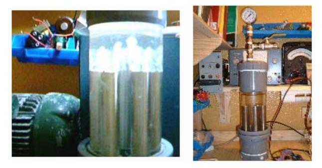
The electrolysis takes place between each of the inner and outer tubes. The picture above shows the bubbles just starting to leave the tubes after the power is switched on. The picture below shows the situation a few seconds later when the whole of the area above the tubes is so full of bubbles that it becomes completely opaque:
