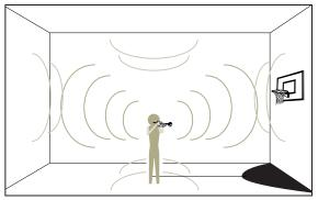
Hard, sound-reflecting surfaces and large cubic volume create excessive reverberation.
